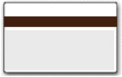
Half Patch use with Mag. Stripe Card Laminate area shown in Grey
